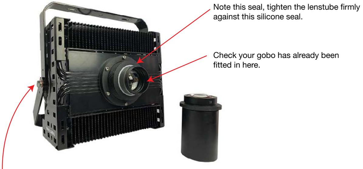
Note this seal, tighten the lenstube firmly against this silicone seal.
