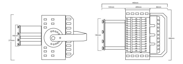
The unit comes with one shutter blade to limit the line length where necessary. Mount the shutter on one side. It wont matter which side because the base mounting plate rotates 360deg to position as required.
