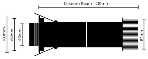
Hole size 86mm minimum, cover plate 109mm
