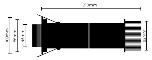
Hole size 86mm minimum, cover plate 109mm
