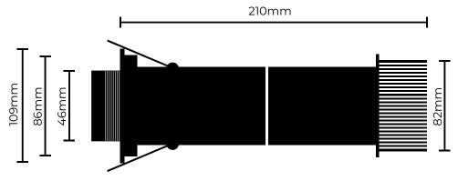
Hole size 86mm minimum, cover plate 109mm
