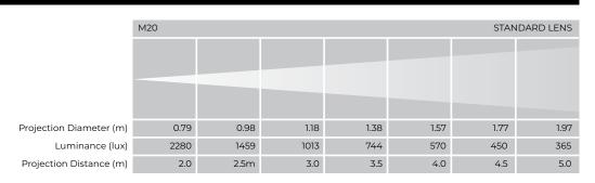
Lux values indicated are not peak values, which may be brighter. We give average lux readings taken under actual tests.
