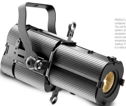
PROFILO LED 80 is a LED-based profile spot contained in a strong and lightweight housing. The unit features an internal four-shutter shaping system, and a 20° to 36° linear zoom. The unit is equipped with a high efficiency 80 W white LED source available with 3000 K or 5000 K color temperature. The unit is suitable for small to medium TV studios, theatres or museums and it is a valid alternative to conventional light.
