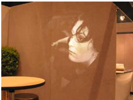
Greyscale images based on photos can be etched into the glass gobo.
